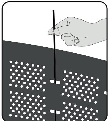
Insert support stakes through the transversal holes to stiffen whole construction.
